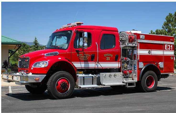
EVFPD Engine 31, a Type 3 wildland firefighting engine. Photo courtesy of EVFPD.
